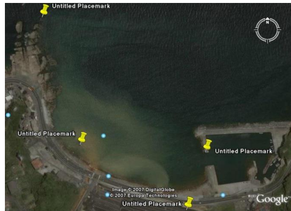
Figure 3. Yellow tacks denote the positions of four GCPs used for geometric transformations
