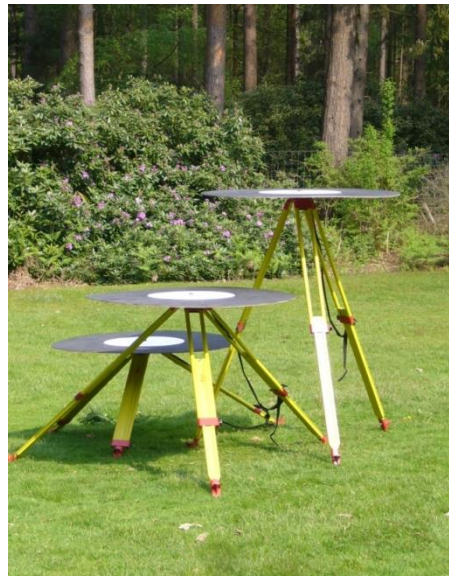
Figure 3. Three lidar targets set at different heights above the ground: 0.6 m, 1.0 m, and 1.6 m.
